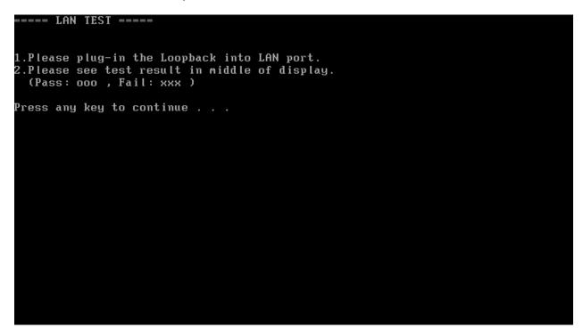
The screen should display as below, indicating whether the subtests pass or fail when finished.
